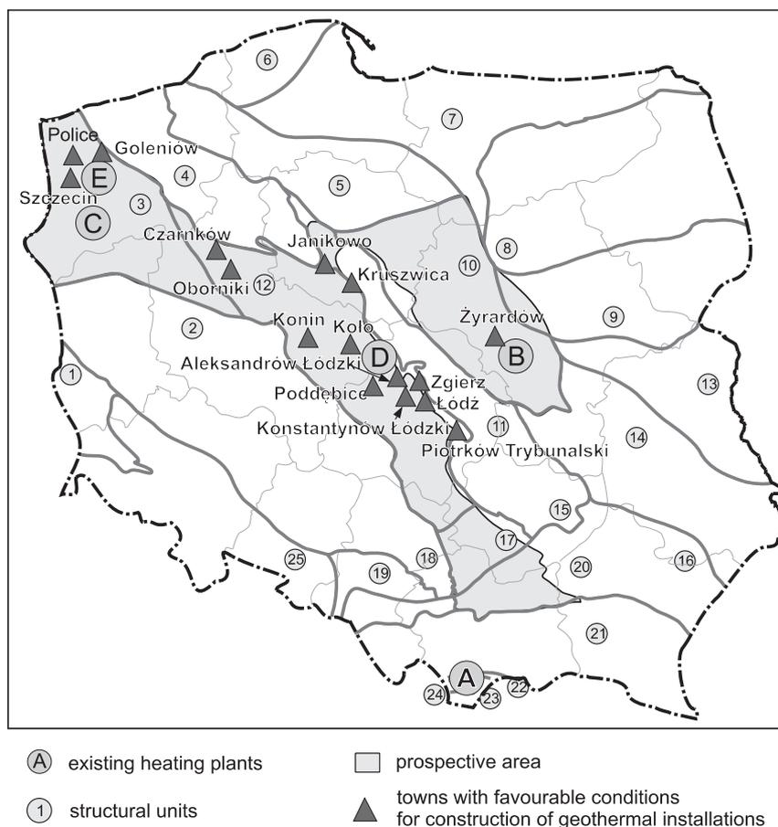
**Fig. 1. Location of towns with favorable conditions for construction of geothermal installations in the Polish Lowlands and existing geothermal heating plants in Poland**
