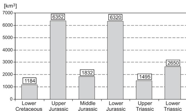
**Fig. 3. Static resources of thermal water within particular geothermal aquifers of Mesozoic age in the Polish Lowlands**
