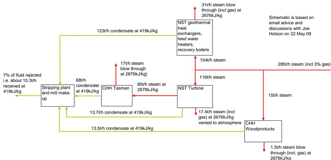
**Figure A3.2: Additional Detail Focussed on Rejected Heat within the Mill Complex**
