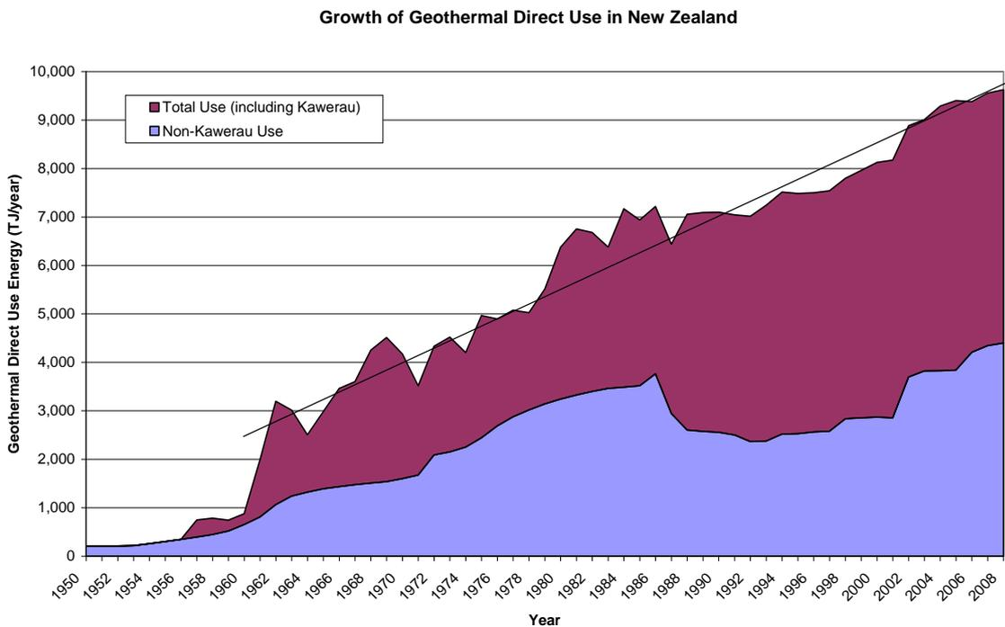
**Figure 2: Historical growth of geothermal direct use (consumer energy) in New Zealand**
