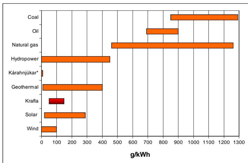
Table 1. CO<sub>2</sub> emission and total running capacity of power plants divided into 9 emission categories (International Geothermal Association (2002))
