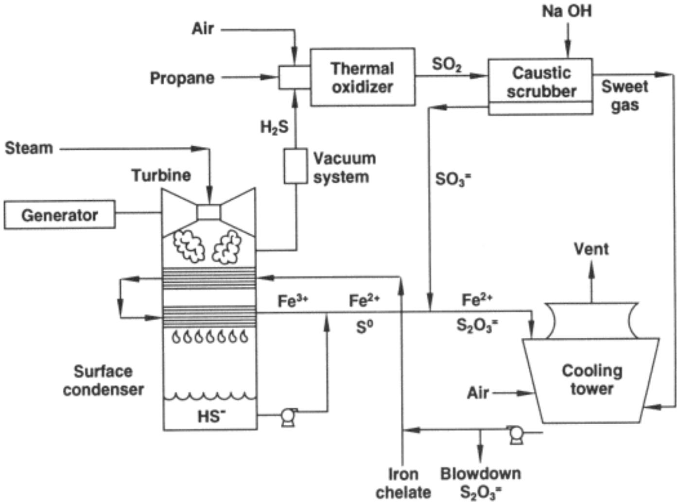
**Figure 2.** Equipment used in the incineration process for hydrogen sulfide abatement at The Geysers geothermal field. (From Bedell, S. A. and Hammond, C. A., *Geothermal Resources Council Bull.*, 16, 3, 1987, with permission.)
