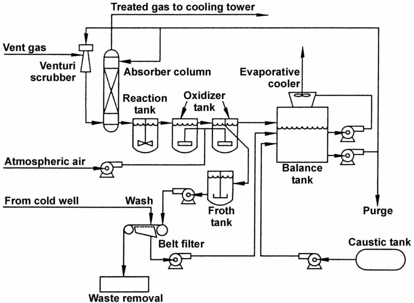
**Figure 1.** Typical equipment used in the Stretford process for hydrogen sulfide abatement at The Geysers geothermal field. (from Henderson, J. M. and Dorighi, G. P., *Geothermal Resources Council Trans.*, 13 593, 1989, with permission.)
