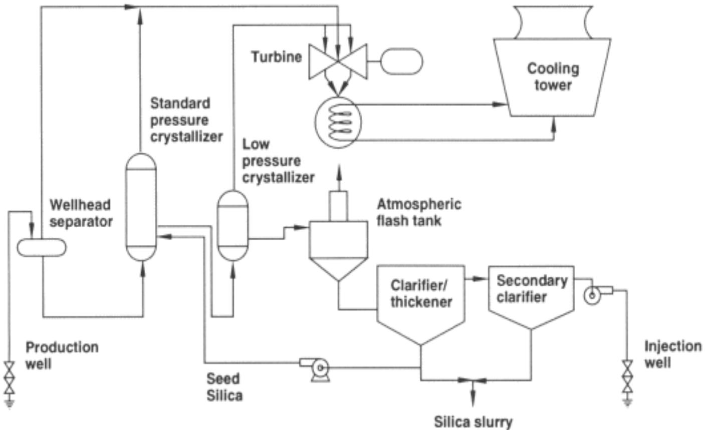
**Figure 3.** The flow stream for removal of solids from the vapor and brine in typical power plants in the Salton Sea geothermal field. (From Signorotti, V. and Hunter, C. C., *Geothermal Resources Council Bull.*, 21, 277, 1992, with permission.)
