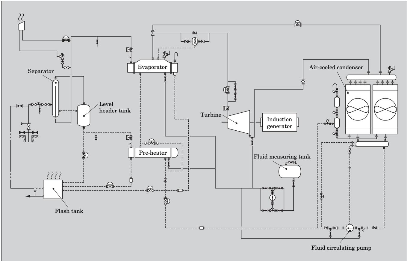
Fig.3 Overview of prototype system
