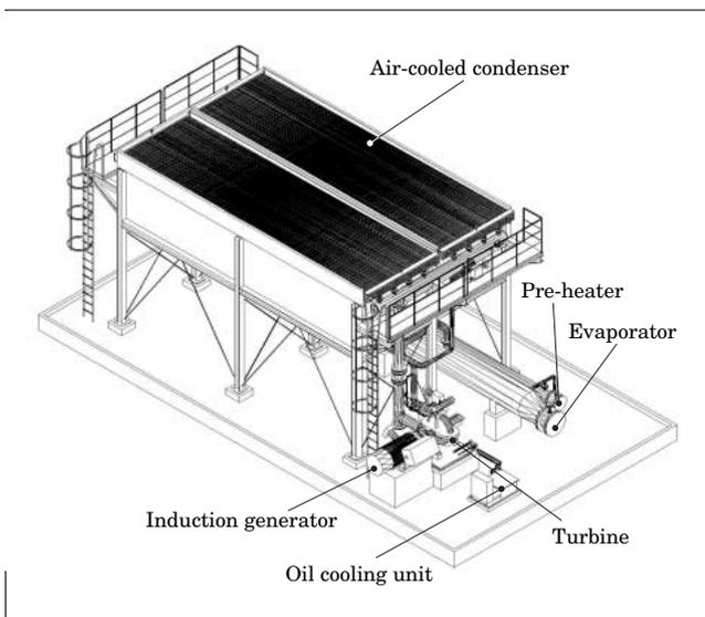
fore, a standard single-stage steam turbine is utilized. However, a dual mechanical seal system is applied at the shaft seals to eliminate any leakage of iso-pentane from the shaft ends.
