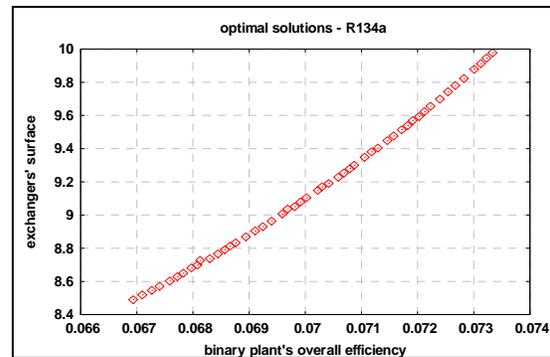
Fig. 1. Rankine cycle optimization - optimal solutions for R134a.
