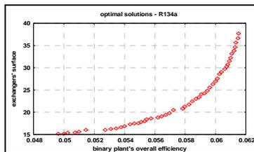
Fig. 3. Rankine cycle optimization- optimal solutions for ORC machine B.
