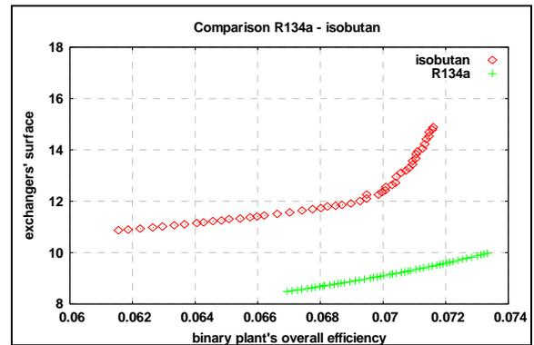
Fig. 2. Rankine cycle optimization- optimal solutions for both R134a and R600a.
