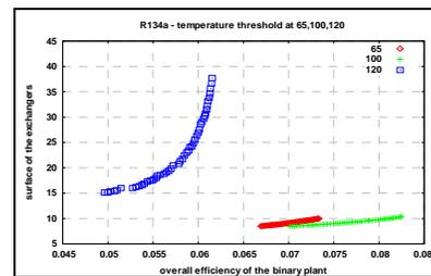
Fig. 4. Rankine cycle optimization- optimal solutions for R134a machines.
