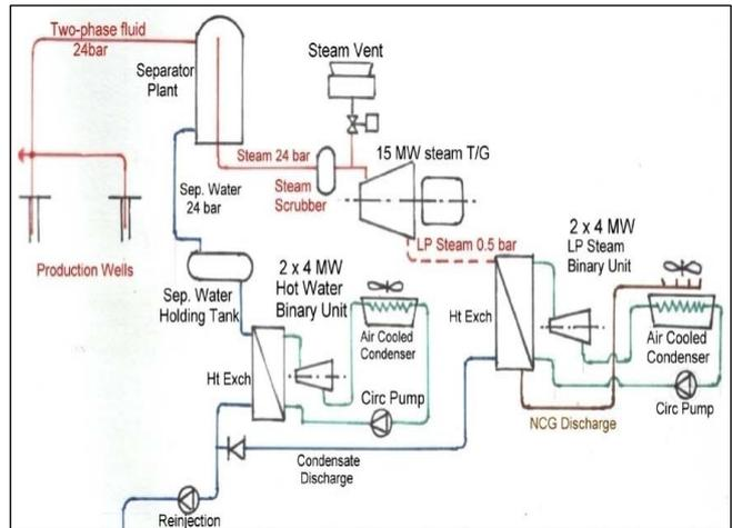
Fig. 5 - Hybrid geothermal power plant (Thain, 2009)
