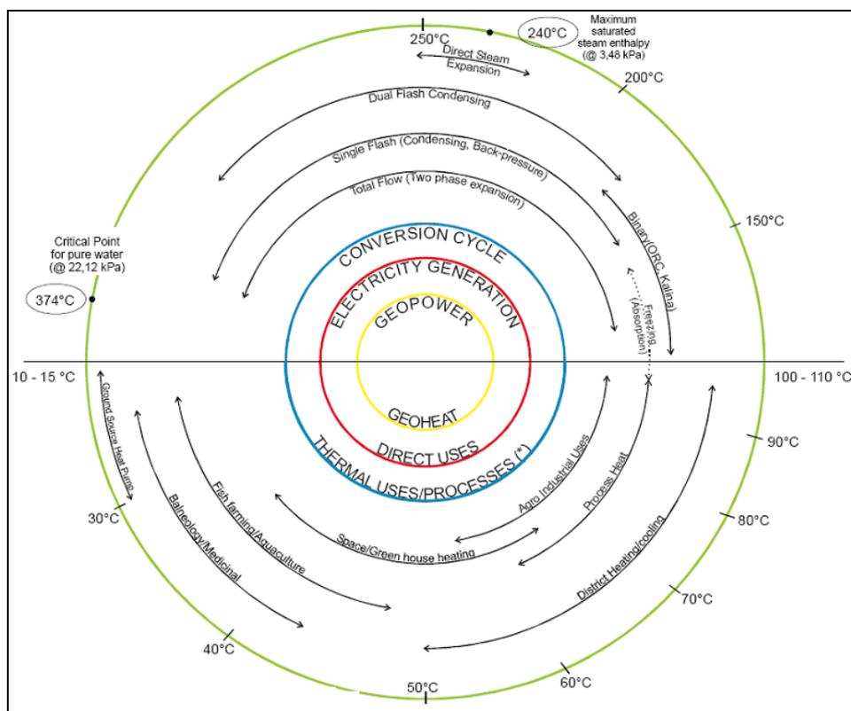
Fig. 1 - Geothermal resource utilisation potential (Antics and Ugemach, 2009)
