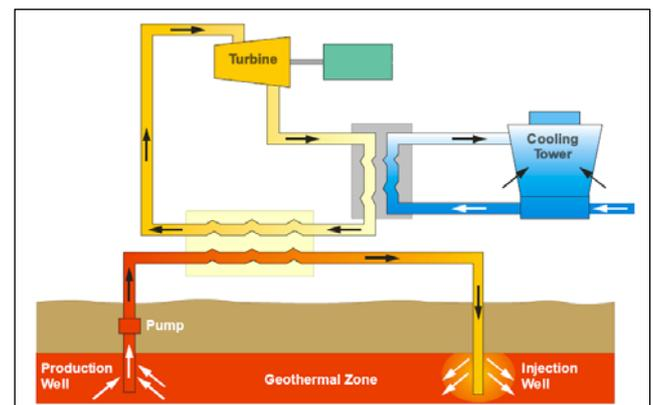
Fig. 4 - Binary cycle geothermal power plant (Kutscher, 2004)
