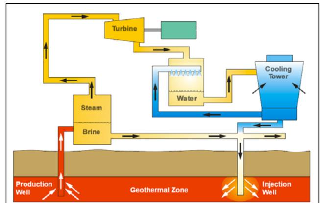
Fig. 3 - Flash geothermal power plant (Kutscher, 2004)
