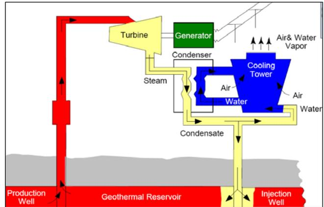
Fig. 2 - Direct steam geothermal power plant (Sanner, 2007)
