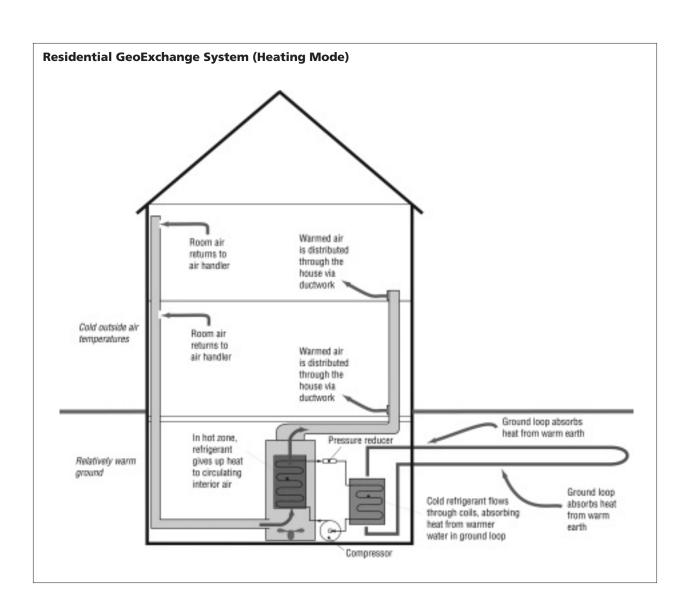
In both cases, a pump circulates liquid through the *loop* and the *heat pump*. The *heat pump* chills (or collects the heat stored in) the liquid when it is being used as a source of heat, and circulates it back through the *loop* to pick up more heat. A system for a large home will require a larger heat pump and ground loop, with a circulation pump to match.
