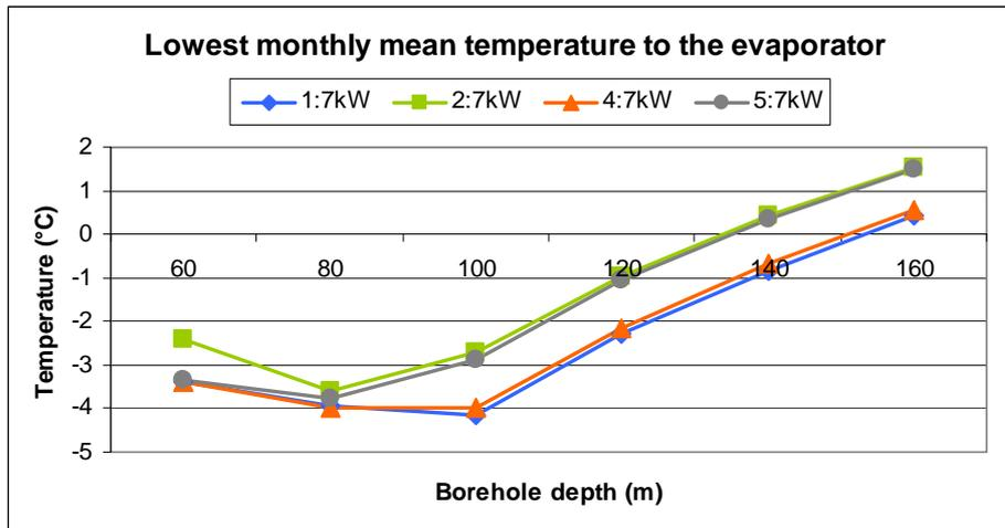
Figure 2: Lowest monthly mean temperature to the evaporator with different depth of boreholes, for four different systems for boreholes 60 – 160 m.
