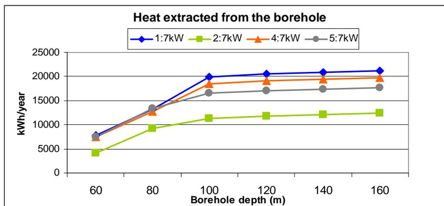
Figure 5: Heat extracted from the ground for the four systems, for boreholes depths 60 – 160 m.
