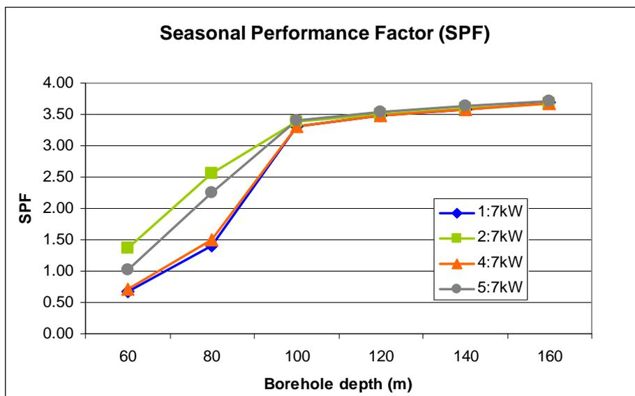
Figure 3: Seasonal performance factor (SPF) for the system including auxiliary electricity and electricity to the circulation pumps.
