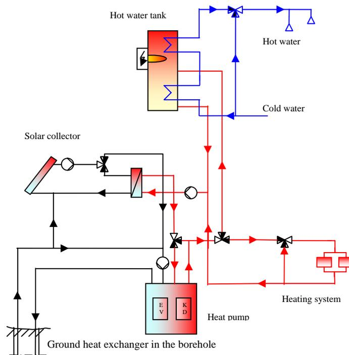
Figure 1: Example of a system with solar collectors in combination with a ground-source heat pump.
