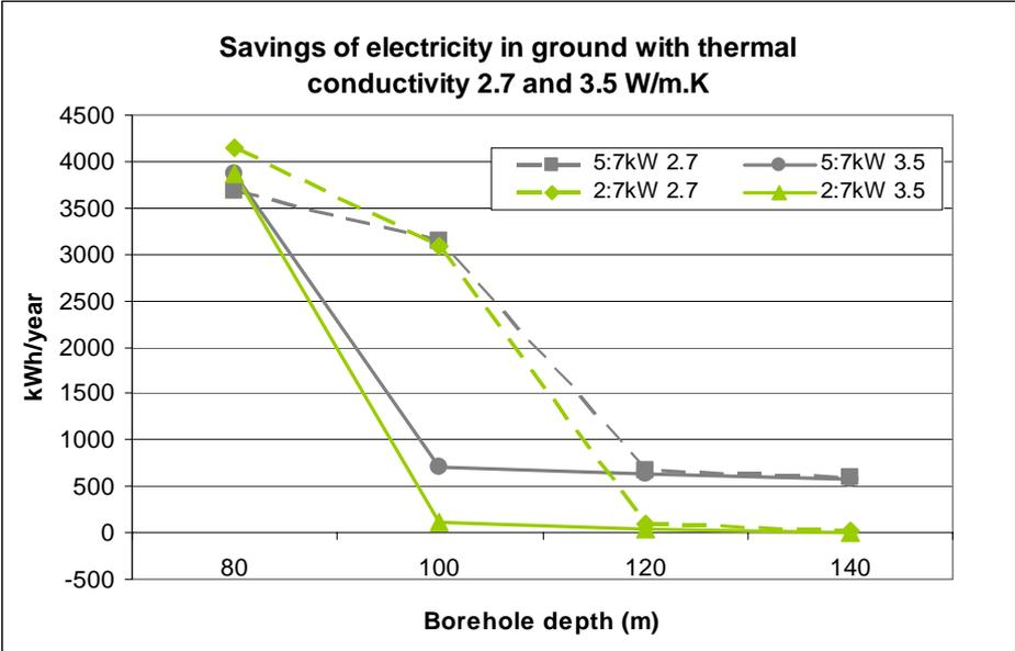
Figure 4: Savings of electricity for systems with solar heat compared to systems without solar heat for two thermal conductivities in the ground, 2.7 and 3.5 W/m,K respectively.
