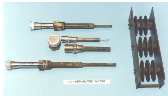
Figure 6. ER probe result for carbon steel in separated water.
